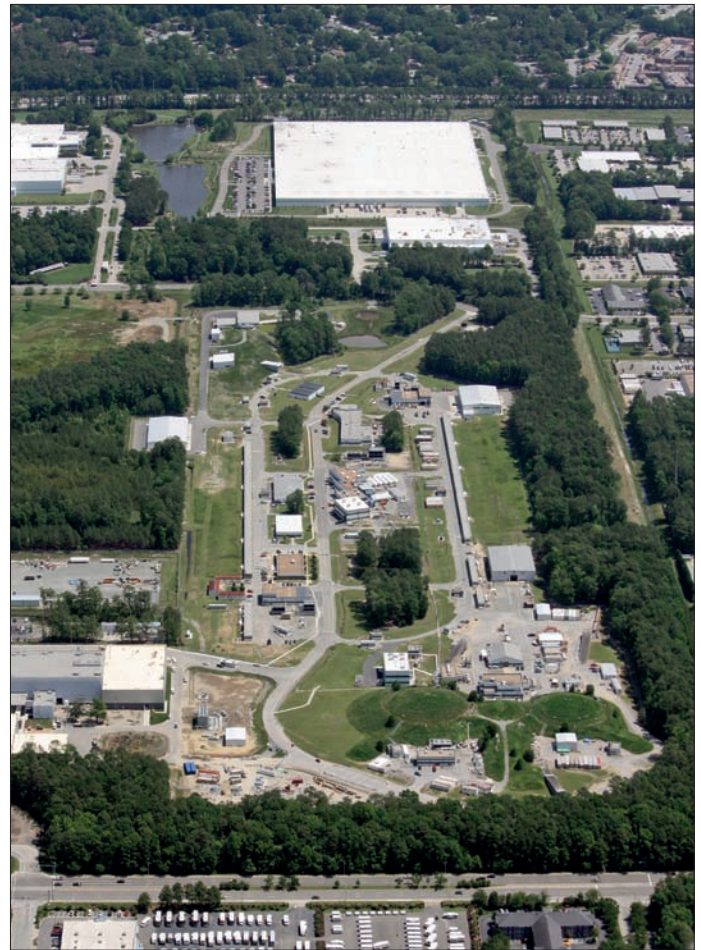
The CEBAF accelerator site is fully visible in this aerial photo, taken in May 2012. The outline of the racetrack-shaped accelerator is at the centre, with the circular experimental halls A, B and C in the bottom right corner and the rectangular Hall D just beyond the racetrack at the top left.
