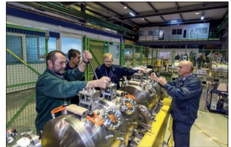
Top: Final module assembly of the RFQ takes place (left) before delivery to the new Linac4 test stand (right). Bottom: After arrival from Siberia, components for the CCDTL modules are inspected (left) before reassembly (right).
